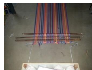
Plate 7: Smaller warp groups attached to the new weighted box
