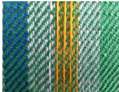
Plate 11: Undesirable warp floats
