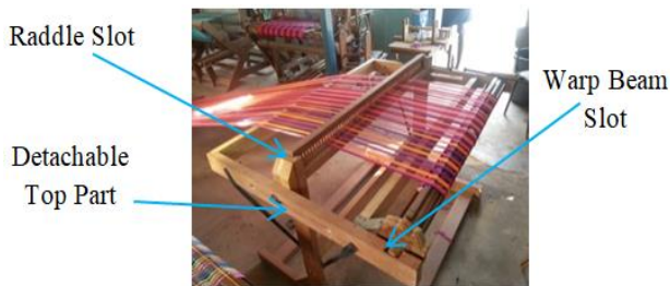
Plate 3: Beaming on the Beaming Device
