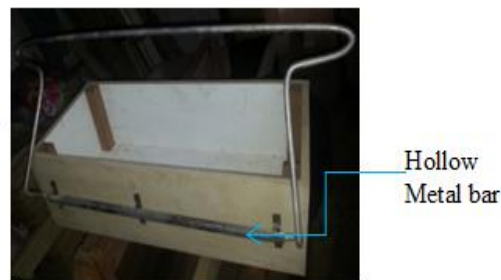
Plate 9: The metal rod attached to the hollow bar
