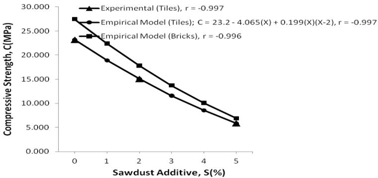
Figure 4: Compressive Strength,  $C$  versus Sawdust Additive,  $S$
