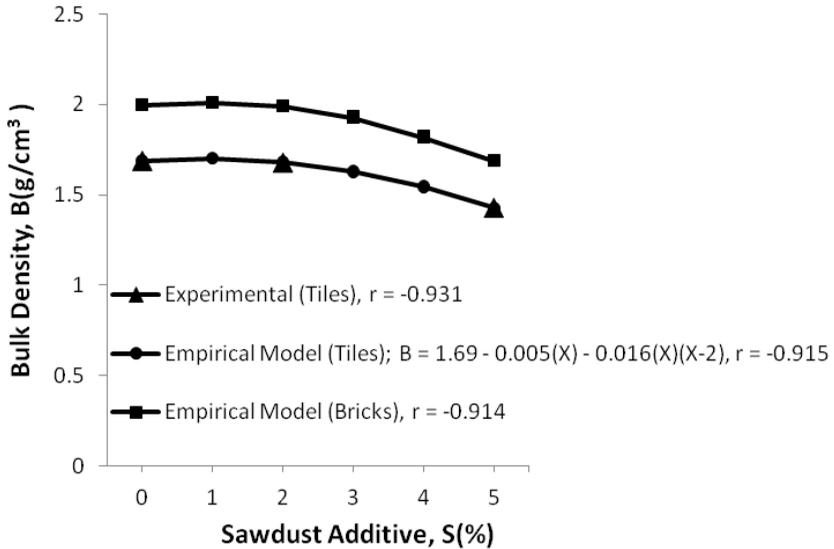
Figure 2: Bulk Density, B versus Sawdust Additive, S
