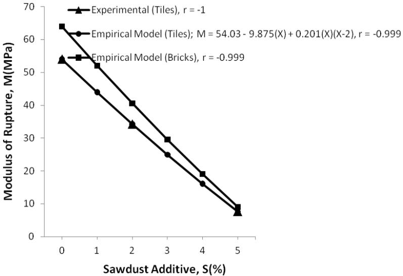
Figure 3: Modulus of Rupture,  $M$  versus Sawdust Additive,  $S$
