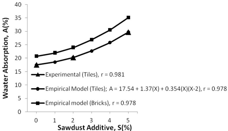
Figure 1: Water Absorption, A versus Sawdust Additive, S
